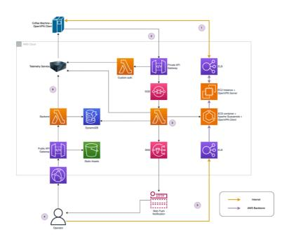
When an operator installs a new machine, they register it through the web app, which registers it into the OpenVPN server and sends the VPN profile to the telemetry service.
