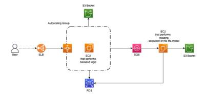
To start off, we should separate our website and backend logic from our machine learning algorithm logic and image resizing logic in order to improve efficiency and streamline our processes. This will allow us to better manage the different tasks and ensure that each component operates optimally.
