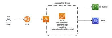
To manage an increasing number of users, we need to scale our architecture for better performance. Our solution is to use an Elastic Load Balancer with an Autoscaling Group to increase the number of EC2 instances computing the images.
