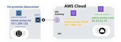
We can also use different DNS subdomains, delegating the subzone to a DNS server that can maintain the configuration for the selected environment. In this scenario, our on-prem development environment will be on the *acme.int* DNS zone for our on-premise datacenter and *cloud.acme.*int for the testing environment on the AWS.
