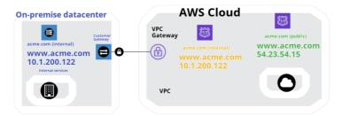
As you can see, www.acme.com address would be different in the AWS Cloud VPC and on the internet, so internal services will be available only through the VPN connection with the proper web server configuration (using rules and ACLS).
