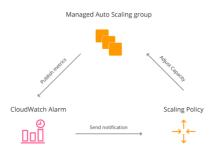
If an instance belongs to an Auto Scaling group, its lifecycle differs from other EC2 instances' one. EC2 Auto Scaling Lifecycle is well illustrated in the following scheme.
