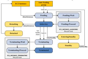
When a new instance is **launched in response to a scale-out event,** it first enters the **Pending state.** This state is designed to allow you to configure (preferably automatically) the EC2 instance and to check its healthiness before moving into the InService state. While into the InService state, the EC2 instance can potentially move **to one of the following three states:**
